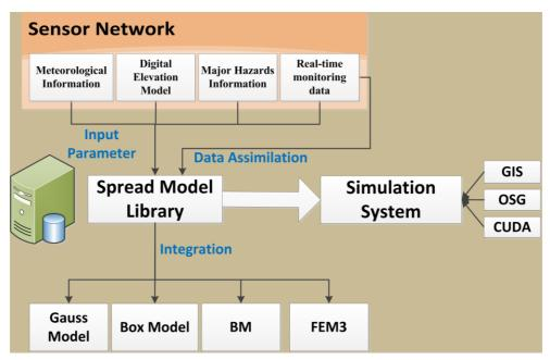
Figure1. Main Components of the System
