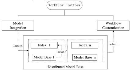
Figure 1. The mechanism of model sharing on a grid workflow platform
