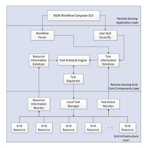
Figure 2. The architecture of the task scheduling sub-system for RSSN platform.
