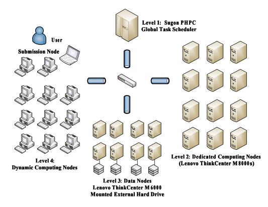
Figure 1. The physical architecture of the RSSN platform.
