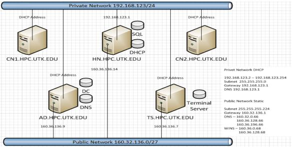
Figure 1. The configuration of MSHPC environment.
