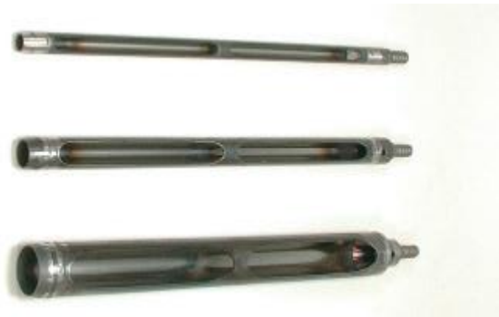
Figure 3. Percussion Gauge Core sampler
