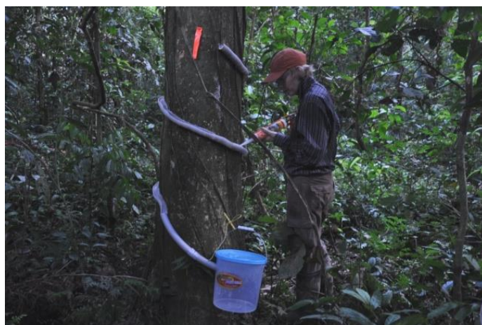
Leena Vihermaa attaching the stem flow collection system on a tree. Samples of stem flow were collected for DOC analysis immediately after rain events and the total volume determined.
