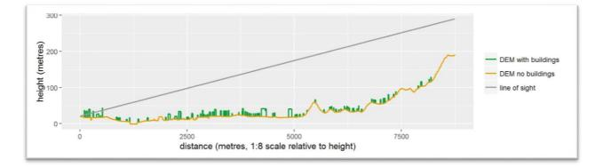
Figure 4: example line of sight blocked by buildings that would not be blocked by landscape alone. Matches dotted line in above figure. Property on left, Cathkin Braes turbine tip on right. Note horizontal distance is 1/8 of actual scale, relative to height.
