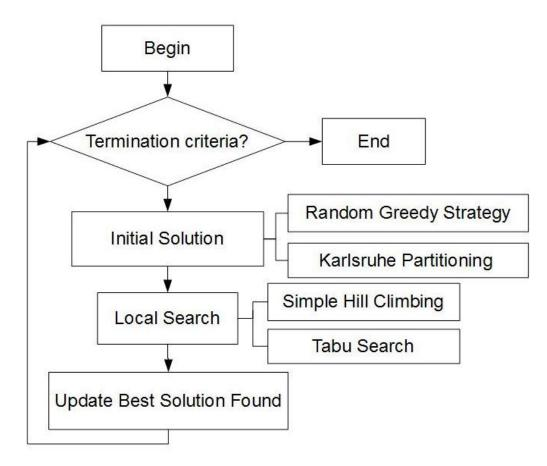
Figure 1. Flowchart of the algorithm for SNPDP
