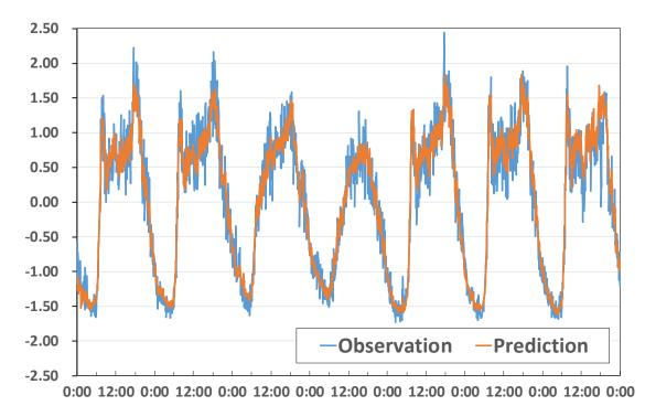
Figure 2: Traffic volume observations and predictions by Model  $A_3$  for street VICS ID #17 from September 1 to September 7.
